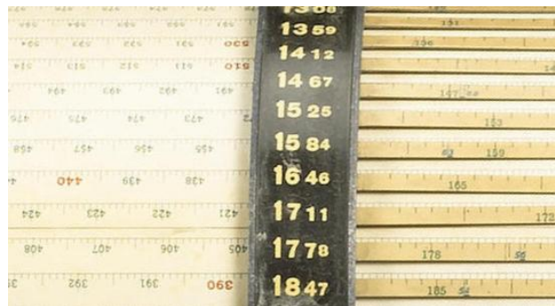
Figure 14: Detail of a 15m LOGA cylindrical slide rule, with the grid wrongly mounted. ( http://www.bonhams.com/auctions/13633/lot/249 )
